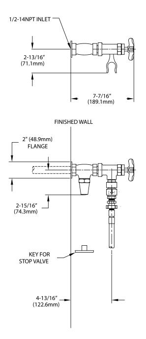
1/2" NPSM Female Inlets Operating Temperature: 40 - 180°F (5 - 83°C) Operating Pressure: 15 - 125psi
